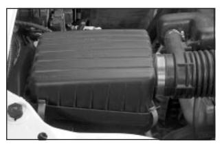
See Engine Compartment Overview on page 5-12 for location of engine air cleaner/filter.
